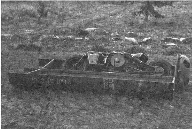
Figure 3 - Welbike Mark I motorcycle in a CLE MkI airdrop container (IWM H 27061)
