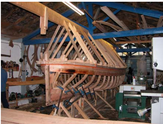
The frame of a copy of a traditional Basque boat (above) The Y shaped pieces of wood are used at the base of the boat at the front
