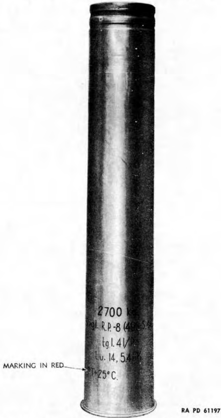
Figure 72 – German 88-mm Cartridge Case, Showing Stenciled Markings
