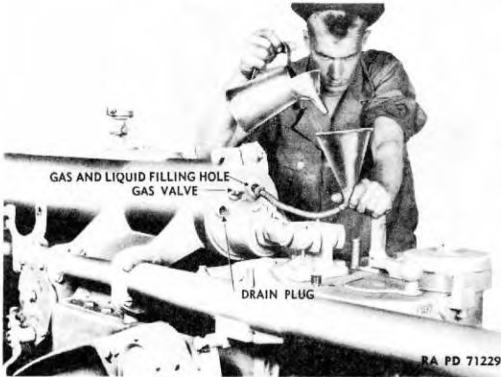
Figure 56 — Filling the Recuperator Cylinder with Liquid
