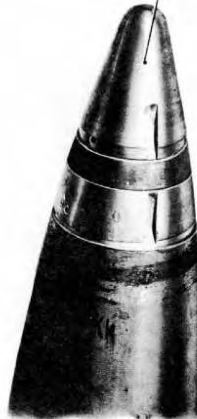
Figure 74 – Spring-wound Time, Percussion, and Inertia-operated Time Fuzes for German 88-mm High-explosive Shell – View Showing Setter Grooves and Selector Element
