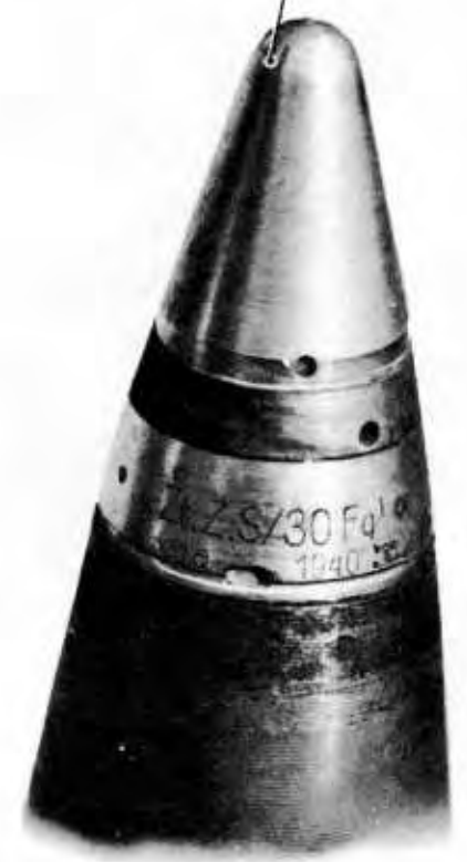
Figure 75 — Spring-wound Time, Percussion, and Inertia-operated Time Fuzes for German 88-mm High-explosive Shell — View Showing Fuze Markings
