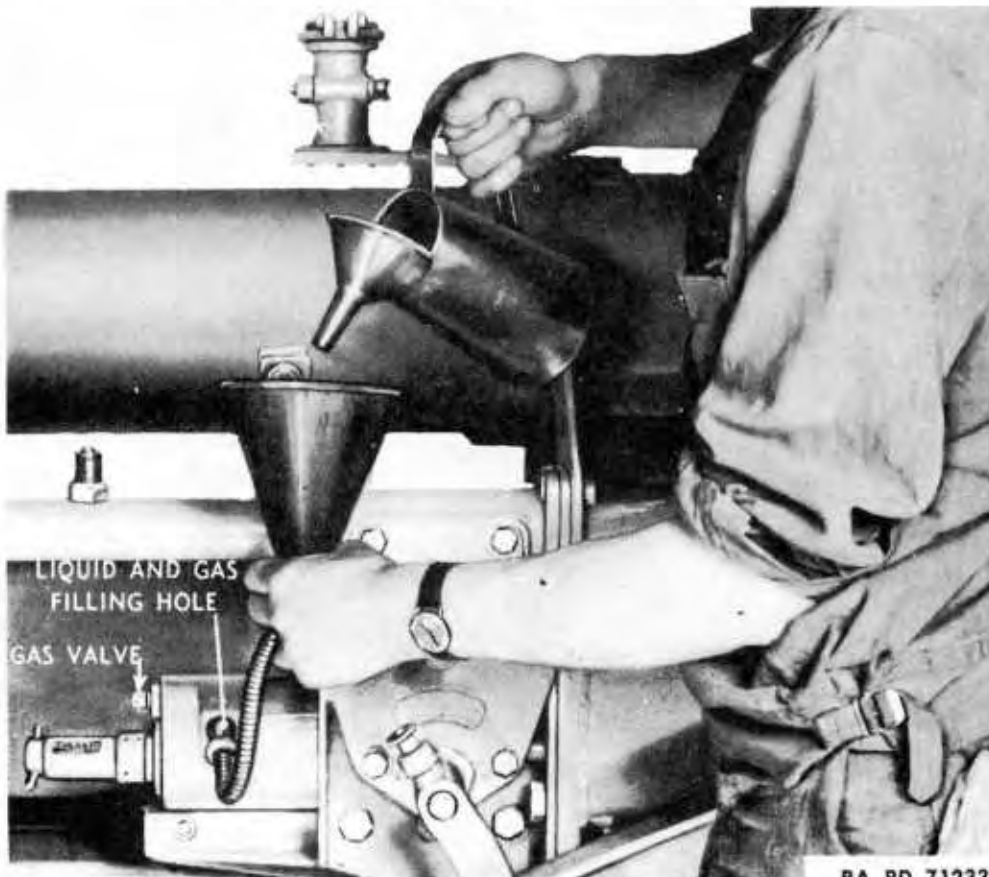
Figure 60 — Filling Rammer Cylinder with Liquid
