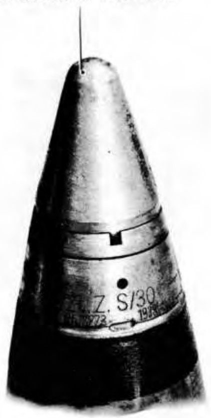
Figure 75 — Spring-wound Time, Percussion, and Inertia-operated Time Fuzes for German 88-mm High-explosive Shell — View Showing Fuze Markings
