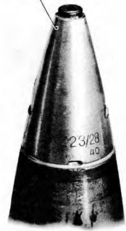
Figure 75 — Spring-wound Time, Percussion, and Inertia-operated Time Fuzes for German 88-mm High-explosive Shell — View Showing Fuze Markings
