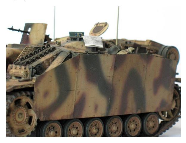
The ALKETT StuG's and StuH's were equipped with a stowage rack fitted to the roof of the vehicle's engine compartment (see the previous picture from the ALKETT factory). The stowage rack for these ALKETT vehicles wasn't a field modification. Unfortunately the stowage rack is also not supplied in the kit.
