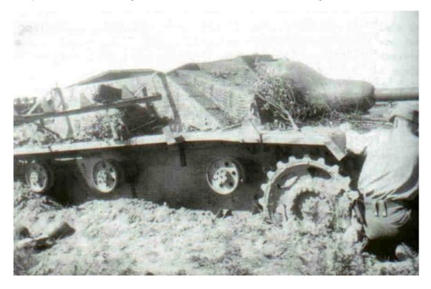
All StuH's of this version had steel return rollers and drive sprockets of the final versions of the StuG G's 1944. The sprockets were actually castings with detachable gear rings. The Dragon kits contains only the 'old' and 'normal' return rollers and drive sprockets. I took the correct return rollers, the drive sprockets and the final drives from the older Dragon StuH kit 9058 that I had in my stash.
