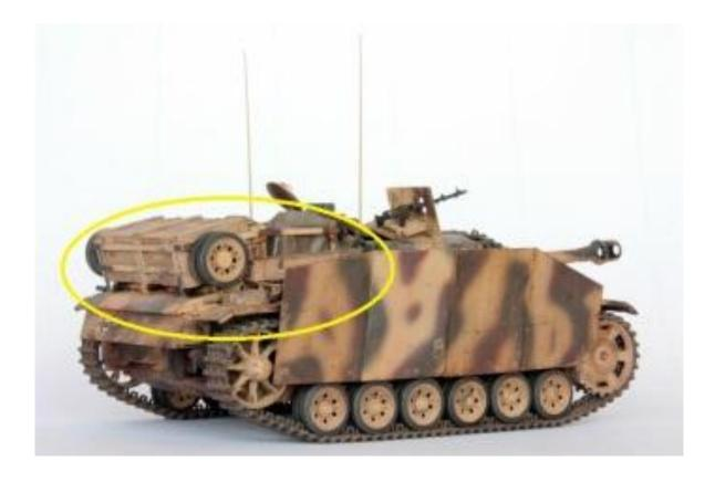
The last small correction I had to make was to fit the correct type of convoy light (Marschlicht) to the rear of the vehicle. Since March 1944 all ALKETT StuG's and StuH's had the new Marschlicht which was a blue glass tube with 4 small lamps in it. If the driver of a following StuG could see all 4 single lamps then the distance between the tanks was to short. If he could see only one broad light then the distance was ok!
