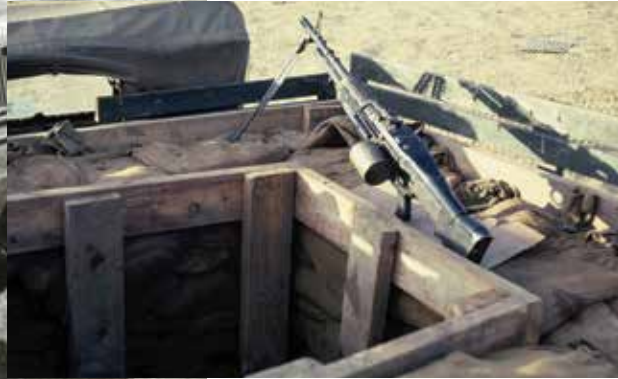
Inside of gunbox created with sandbags and wood walls. M60s were hand held. Photo courtesy of Ted Biggins
