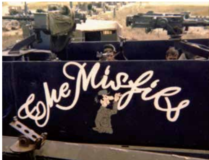
The Misfits had two twin .50s and side mounts for M60s. Photos courtesy of 359th Transportation Company Vietnam
