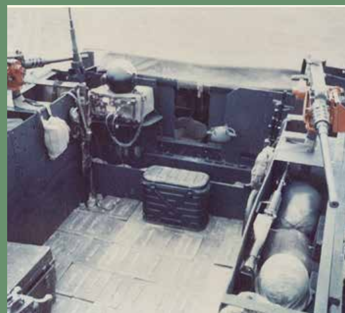
Forward view of the gun box of Eve of Destruction showing radio and side mounted .50s. Cold drinks were kept in the marmite can.
