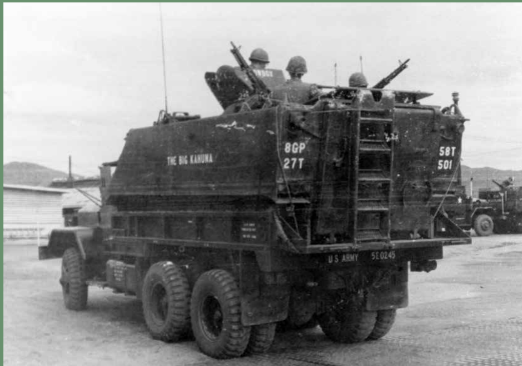
Big Kahuna - Because of the shortage of armor kits, 8th Transportation Group truck companies experimented with sliding M113 Armored Personnel Carrier (APC) hulls on the beds of 5-ton cargo trucks. The APC mounted gun truck was born out of the necessity of finding a way to replace the armor destroyed during a period in which there was a shortage of steel plating in the supply system. Big Kahuna was armed with two M-60 machine guns, one .50 caliber machine gun and one M-79 grenade launcher.
