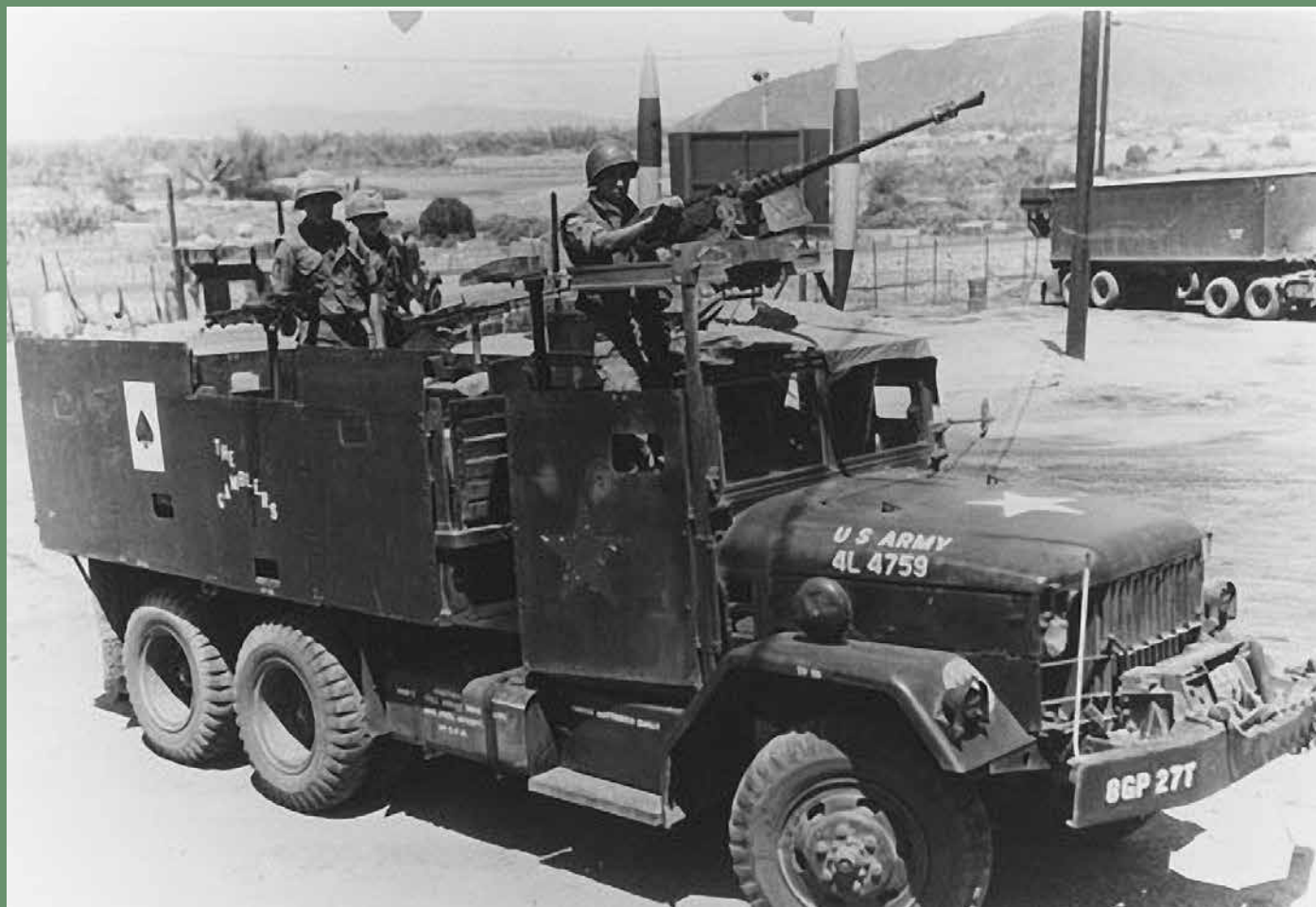
Gambler - Typical 8th Group 2 1/2-ton gun truck with armored plating. This vehicle had sandbagged floors, 2 pedestal-mounted M-60 machine guns with sandbagged emplacements for added protection, and a M-79 grenadier. The vehicle was controlled from ring-mounted .50 cal machine gun. Photos courtesy of the US Army Transportation Museum
