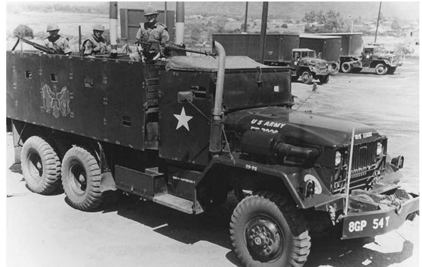
The Hawk - Another version of the versatile gun truck was this M-54A2, 5-ton truck with armored plated cargo bed and cab. The floors and walls had additional sandbag protection. This vehicle was mounted with two M-60 machine guns, a M-79 grenade launcher and .50 cal machine gun. Also, the crew was armed with M-16 rifles and a M-79 grenade launcher. Photo courtesy of the US Army Transportation Museum
